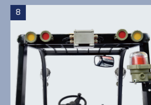
Explosion proof type LED rear work lamp
